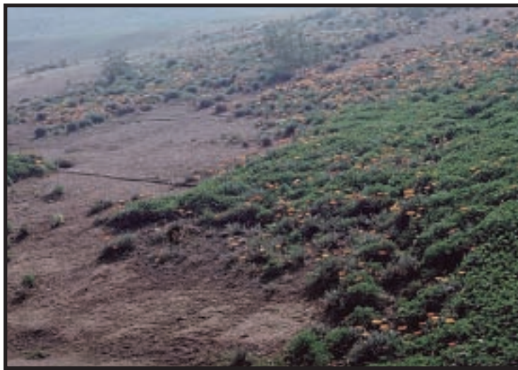
Figure 1. The pH on this cut slope ranged from 3.2, where few plants grew (left side) to 6.2, where growth was normal (right side).
